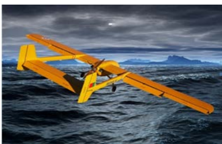
Figure 3 - Portuguese Air Force ANTEX-M UAV used in the SEAGULL project [9].
