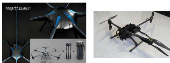
Figure 2 - GammaEX UAVs: a M6 hexacopter on the left and a tricopter on the right [8].
