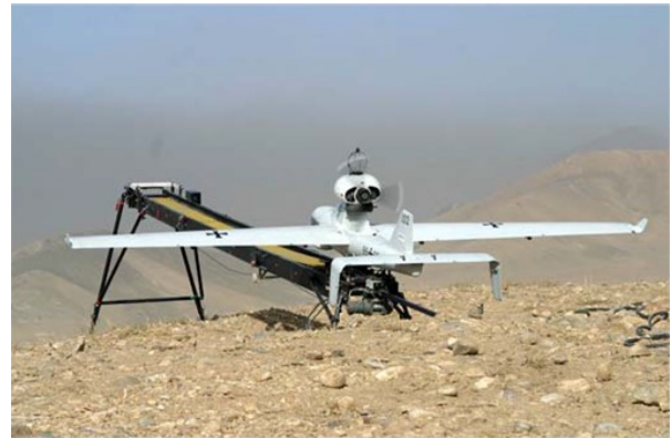
Figure 3 - Bungee Cord launching system [10]
