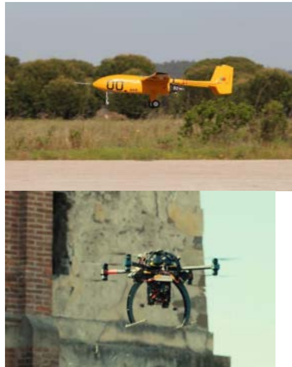
Figure 1: Fixed-Wing (SEAGULL Project) and Multi-rotor (LIFT VI) UAV's
