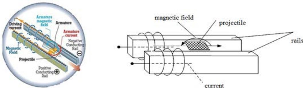
Fig. 3 The operating principle of electromagnetic rail gun
