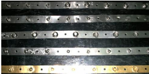
Figure 1: Small cylindrical parts made by cupping with and without willful thinning of sheet thickness
