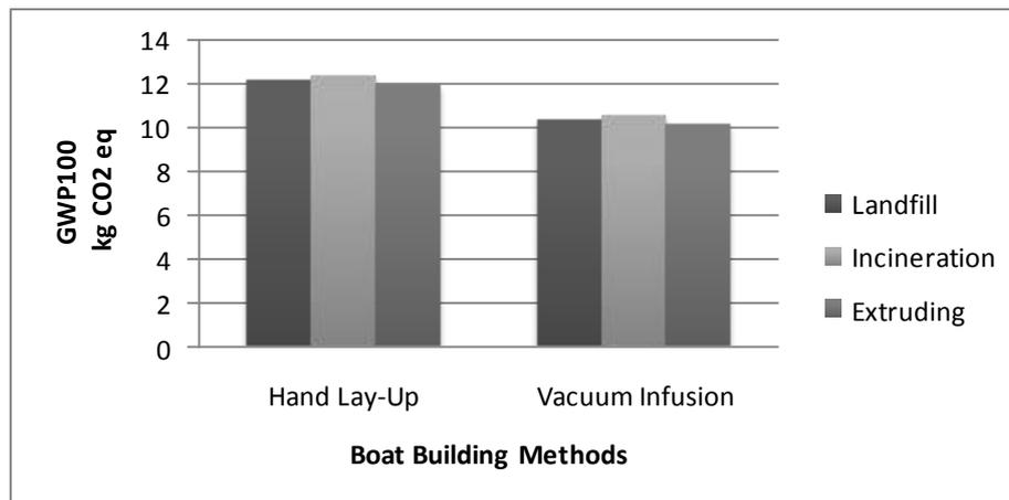
Figure 3 Comparison of GWP<sub>100</sub> results between hand lay-up and vacuum infusion method
