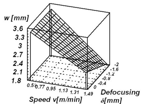
Figure 4 Response surface for weld width measured on weld cross-section with speed and defocus
