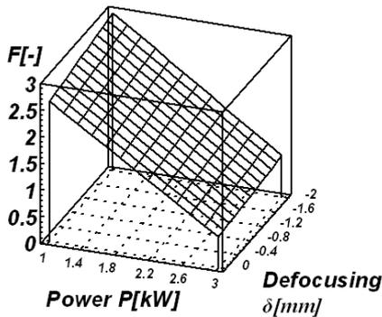
**Figure 7 Response surface for ratio F, depending on power and defocus**
