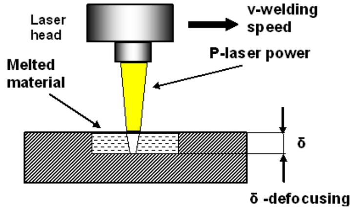
Figure 2 Experimental parameters for welding process
