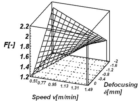
**Figure 8 Response surface for ratio F, depending on speed and defocus**
