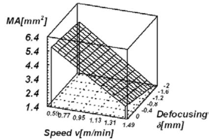
**Figure 10 Response surface for melted area on weld cross-section with speed and defocus**
