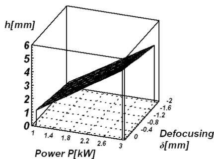
Figure 5 Response surface for weld depth with power and defocus
