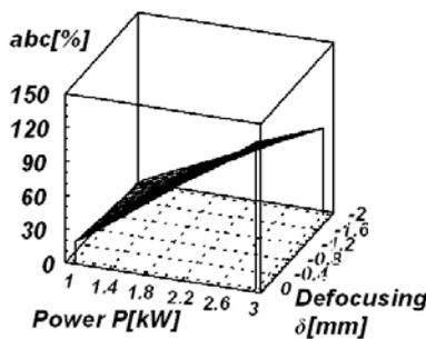
Figure 15 Response surface for crater deformation with power and defocus
