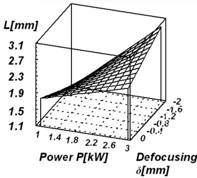
Figure 11 Response surface for average weld width L with power and defocus
