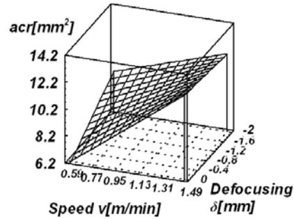
Figure 14 Response surface for crater area, with speed and defocus
