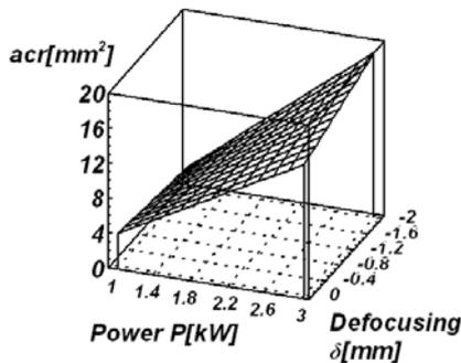
Figure 13 Response surface for crater with power and defocus
