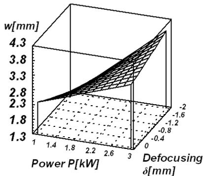
Figure 3 Response surface for weld width measured on weld cross-section with power and defocus
