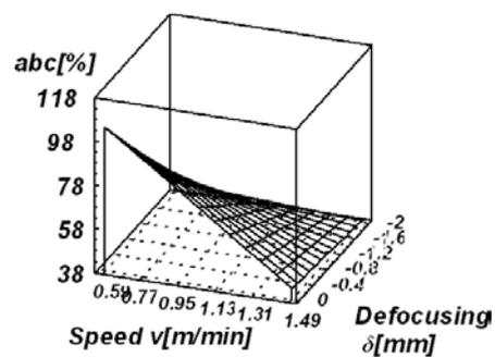
Figure 16 Response surface for crater deformation with speed and defocus
