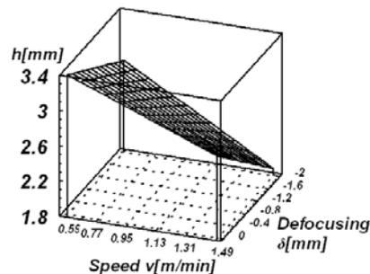
Figure 6 Response surface for weld depth, depending on the speed and defocus
