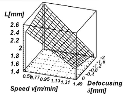
Figure 12 Response surface for average weld width L with speed and defocus
