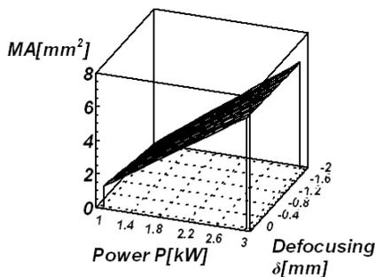
**Figure 9 Response surface for melted area on weld cross-section with power and defocus**
