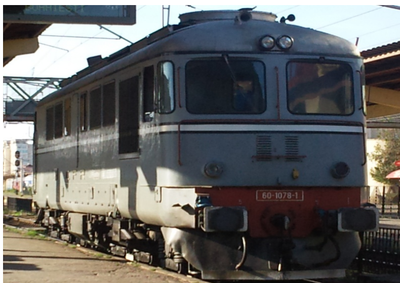
Fig. 1 Diesel-electric locomotive type 060 DA
