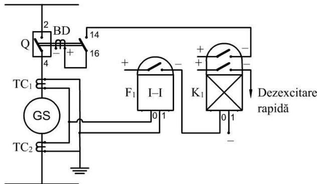
**Fig.1** Single-line electric scheme of a synchronous generator longitudinal differential protection and control. GS- synchronous generator, Q-switch, BD- shutter coil, TC<sub>1</sub>, TC<sub>2</sub>- current transformers, F<sub>1</sub>- current differential relay, K<sub>1</sub>- intermediate relay.
