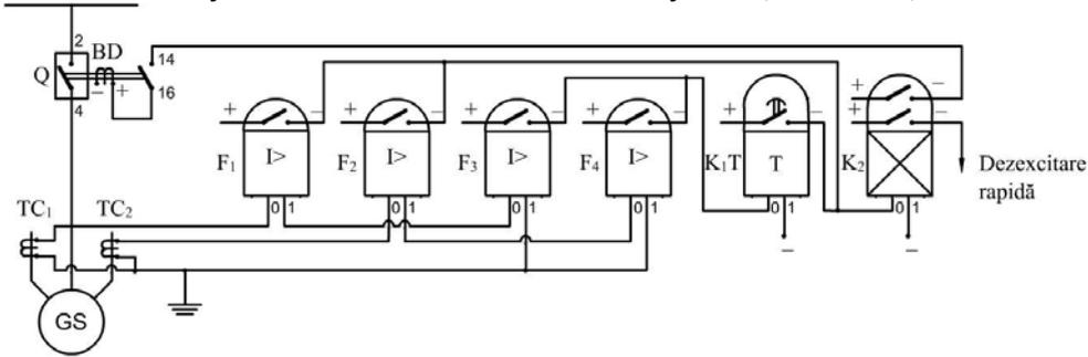
**Fig.19 Synchronous generator protection and control performed with maximal power cut single line electrical diagram. GS-synchronous generator, TC<sub>1</sub>, TC<sub>2</sub>-current transformers, Q -main switch, BD-coil shutter, F<sub>1</sub> ... F<sub>4</sub>-maximum current relay, K<sub>1</sub>T-timing relay, K<sub>2</sub>-intermediate relay.**
