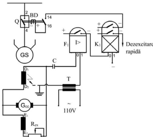
**Fig.2** Single-line electric scheme of protection against short circuits and rotor control. GS-synchronous generator, the main switch Q, BD- shutter coil; Gcc-excitatrice, Rex-excitation rheostat adjustment, the maximum current relay F<sub>1</sub>, K<sub>1</sub> intermediate relay, T-transformer, C-condenser.
