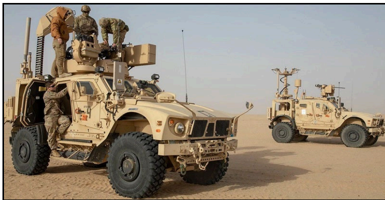
Fig. nr. 10 Sistemul american integrat de combatere a dronelor M-LIDS (Mobile-Low, Slow, Small Unmanned Aircraft Integrated Defeat System) - o posibilă soluție dislocabilă de combatere a dronelor bazată pe tehnologie de bruiaj și lovire / cinetică (Sursa: „M-LIDS – Mobile-Low, Slow, Small Unmanned Aircraft Integrated Defeat System, USA - M-LIDS is a counter-drone capability designed to protect service members and critical assets from enemy drones”, https://www.army-technology.com/projects/m-lids-mobile-low-slow-small-unmanned-aircraft-integrated-defeat-system/ )
