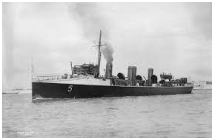
Figure 14. HMS Spiteful - The first warship powered solely by fuel oil – 1899
