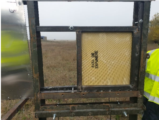
Figure 3.a. The armor support device
