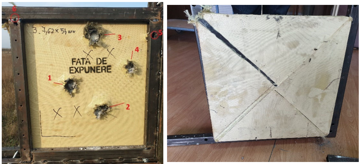
Figure 6. The multilayered armor plate after the 6 bullets firing
