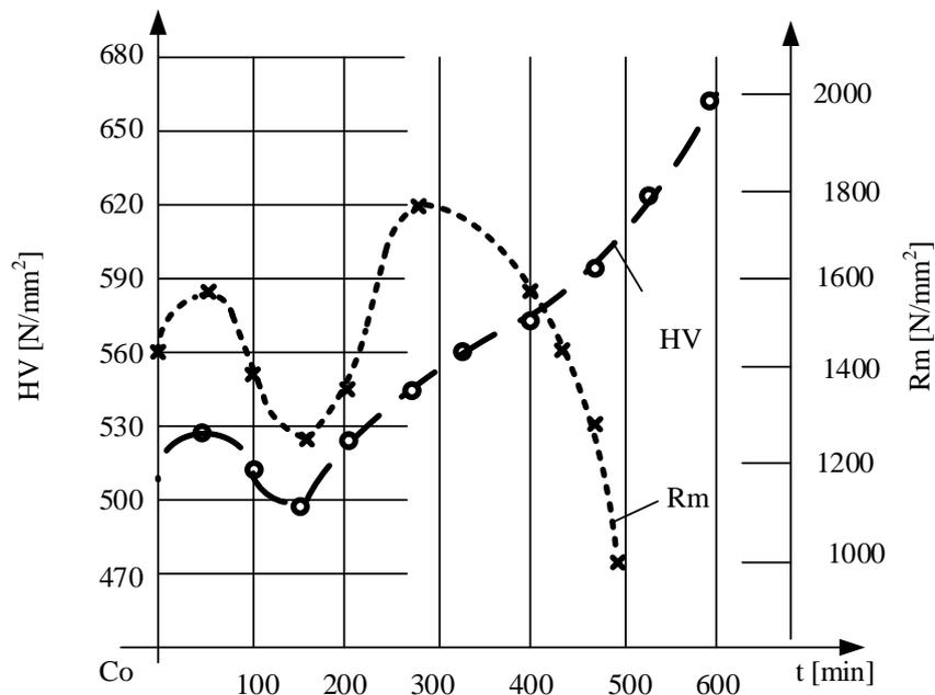
Fig. 2 Influence of aging treatment duration on mechanical strength and Vickers hardness in the case of amorphous metal  $\text{Cu}_{46}\text{Zr}_{54}$
