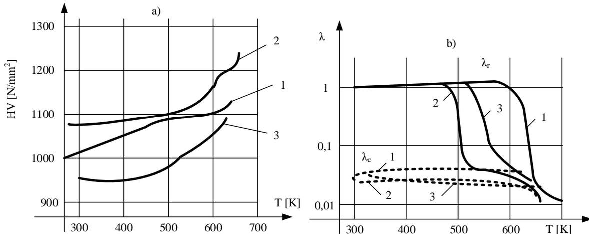
Fig.3 The ductile-brittle transition of amorphous metals from the Fe-Ni-B- (Si) group is highlighted: a) by the variation of hardness; b) by the variation of the deformation at flow and rupture
