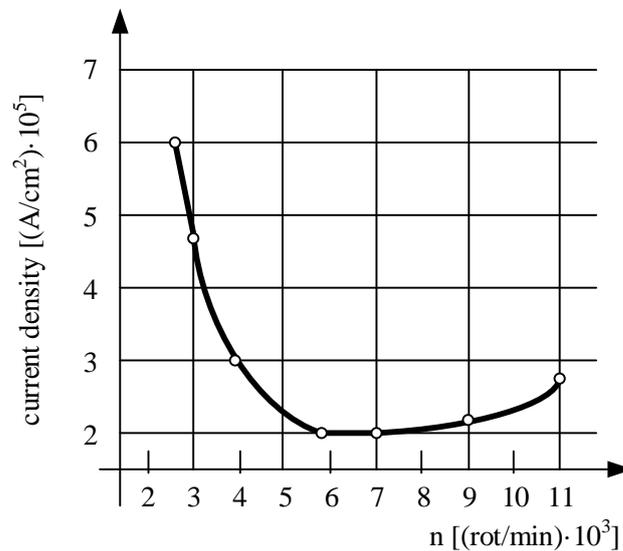
Fig.9 Variation of corrosion resistance depending on the cooling rate of the amorphous metal strip
