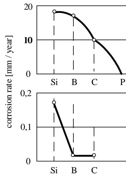
Fig.6 Influence of metalloid content on corrosion resistance of amorphous metal
