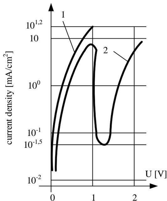
Fig.8 Variation of corrosion resistance of  $\text{Fe}_{80}\text{P}_{14}\text{B}_6$  alloys depending on the metal structure
