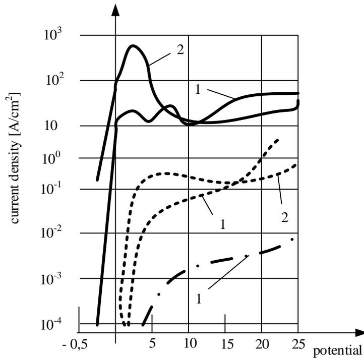
Fig.7 Influence of P on the corrosion resistance of some Ti-Cu alloys with amorphous and crystalline structure
