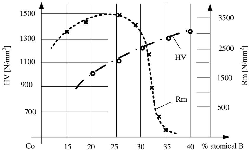
Fig. 1 Variation of mechanical strength and Vickers hardness of amorphous metal in the Co-B system depending on the B content
