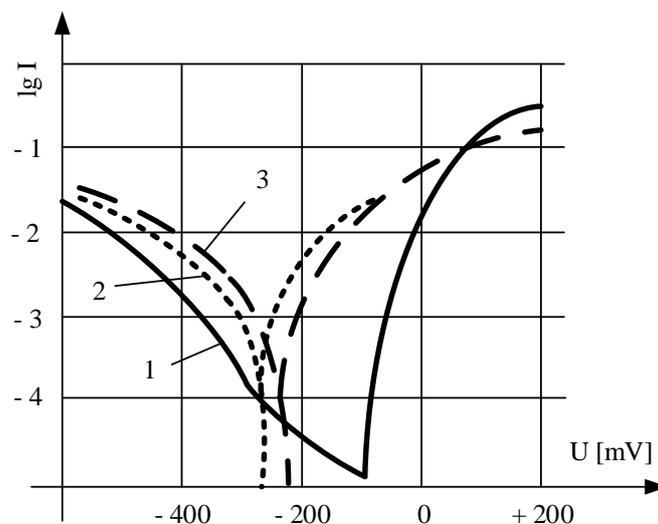
Fig.4 The shape of the polarization curves depends on the type of anions used
