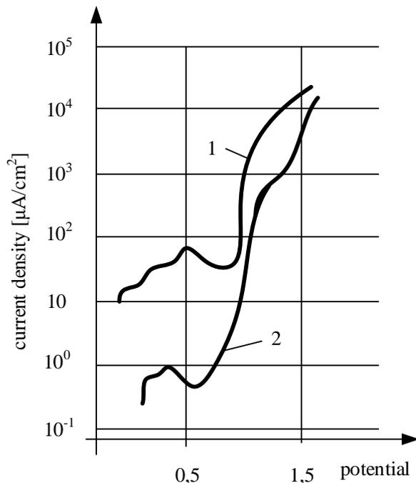
Fig.5 Polarization curves of amorphous metals in the system Fe-Cr-(Ni)-P-C
