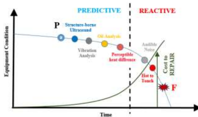
Figure 4. P-F curve for bearing failure in a production system
