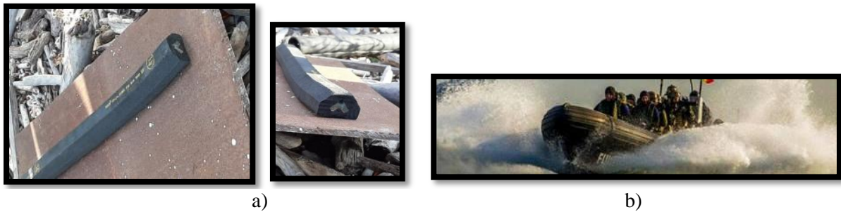
Figure 5. a) Underwater breach creation in metal plates (doors) with flexible cutting blade with cumulative jet, b) transport means, c) divers carrying the initiation device, d) the underwater explosion and, e) the effect obtained underwater, f) measuring and noting of the effect obtained under water.
