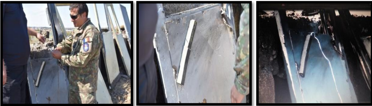
Figure 3. a), b), c) Creation of breach in metal door with flexible load with BLADE type cumulative jet
