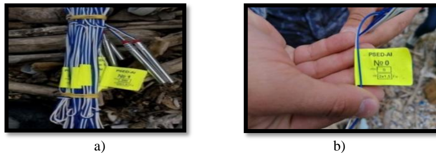
Figure 6. a) Detonating electrical staples (CED) with delay and b) without delay
