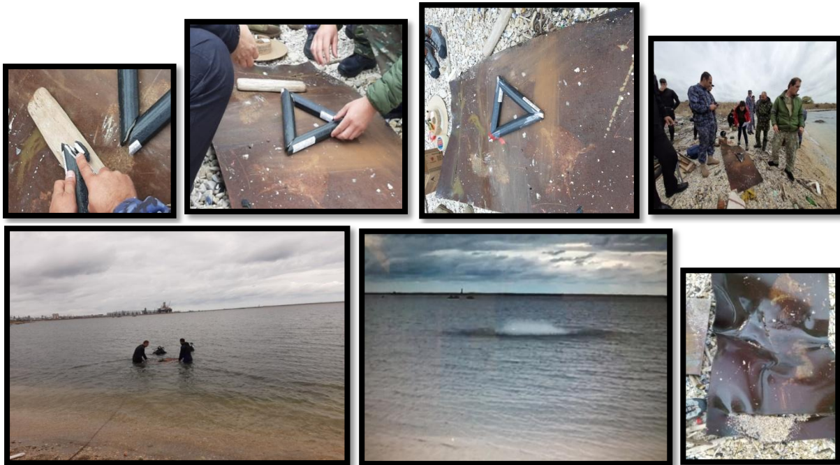
Figure 8. Underwater cutting on the contour of a 10mm thick naval sheet with DES made of jet flexible load / ICTRM 10 cumulative effect type (made at UPS Dragomirești) combined at the corners with HITEX type explosive (produced at UPSD) and the effect obtained
