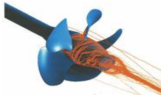
Figure 3. Formation of the hub vortex behind a navy propeller equipped with a special hub cap
