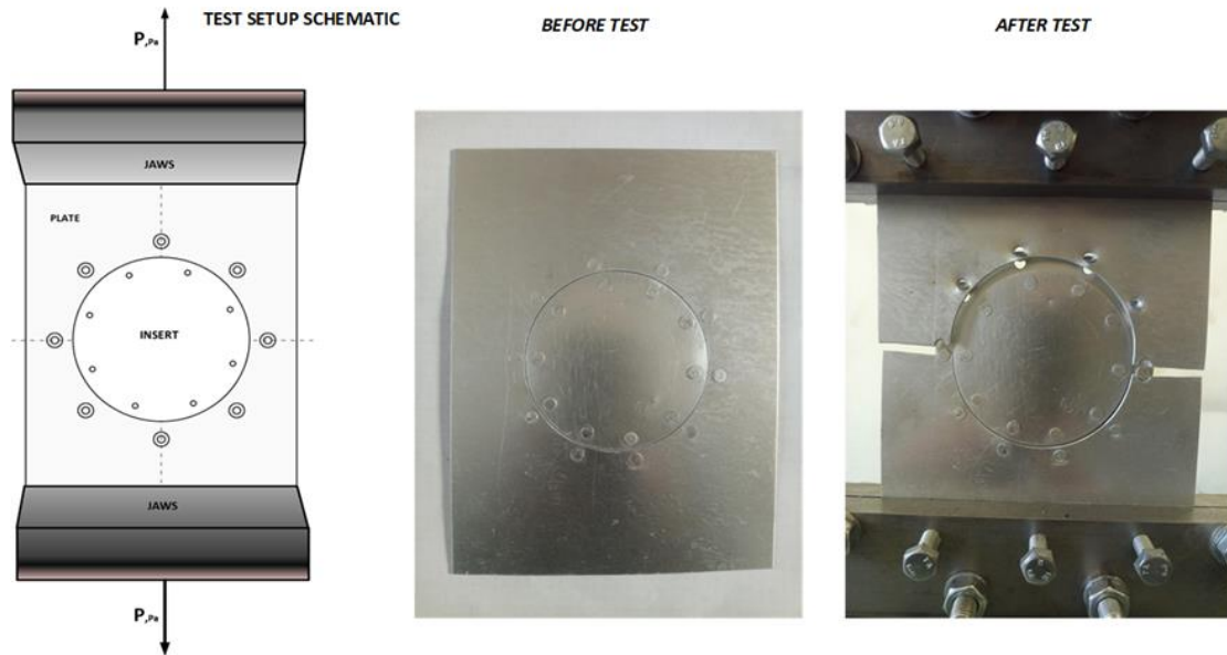
Figure 4. Schematic diagram of the test and photographs of the already destroyed samples
