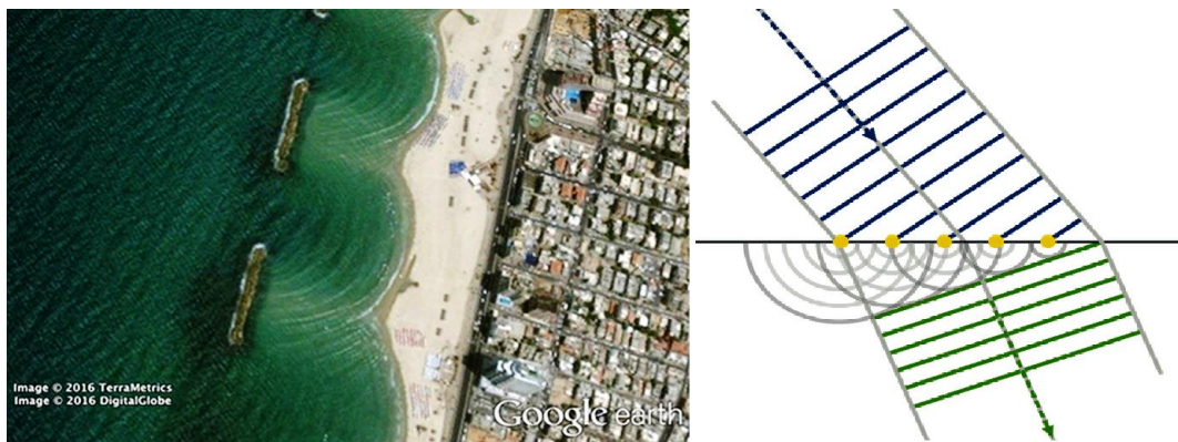
Figure 10. The wave diffraction phenomenon [10]
