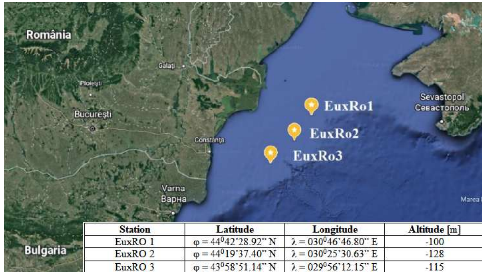
Figure 5. Positioning of EuxRo autonomous marine monitoring stations on the Romanian continental platform [8]
