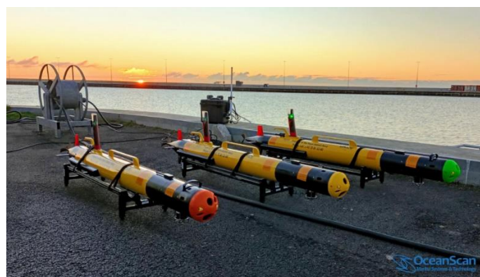
Figure 9. OCEANSCAN-MST LAUV (Light Autonomous Underwater Vehicle) units with integrated Voyis technology [18]
