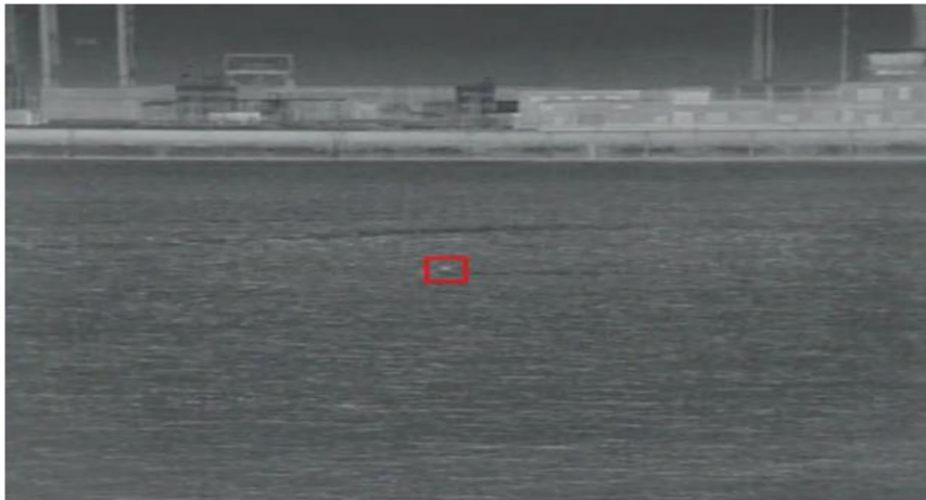
Figure 5. Drifting mine in the port of Zeebrugge, captured by the MicroCompass MWIR sensor on the P901 Castor [7]
