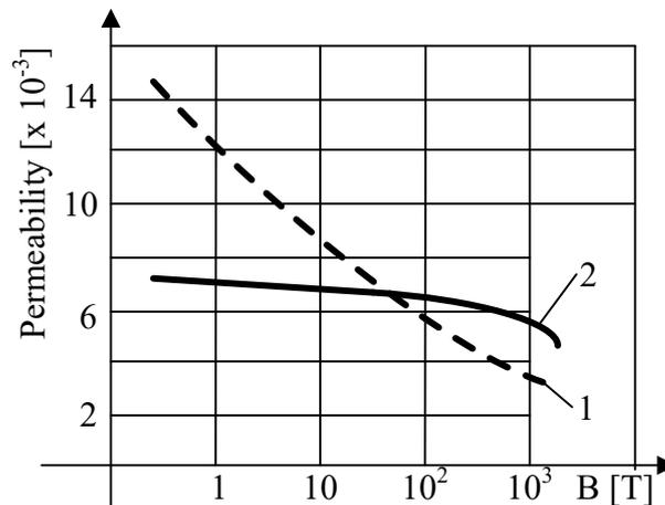
Fig. 5 Variation of magnetic permeability as a function of cooling rate during aging of an amorphous metal [9]
