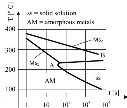
Fig. 6 General shape of a TTT diagram for metal-metalloid type amorphous metals ([1], [5])
