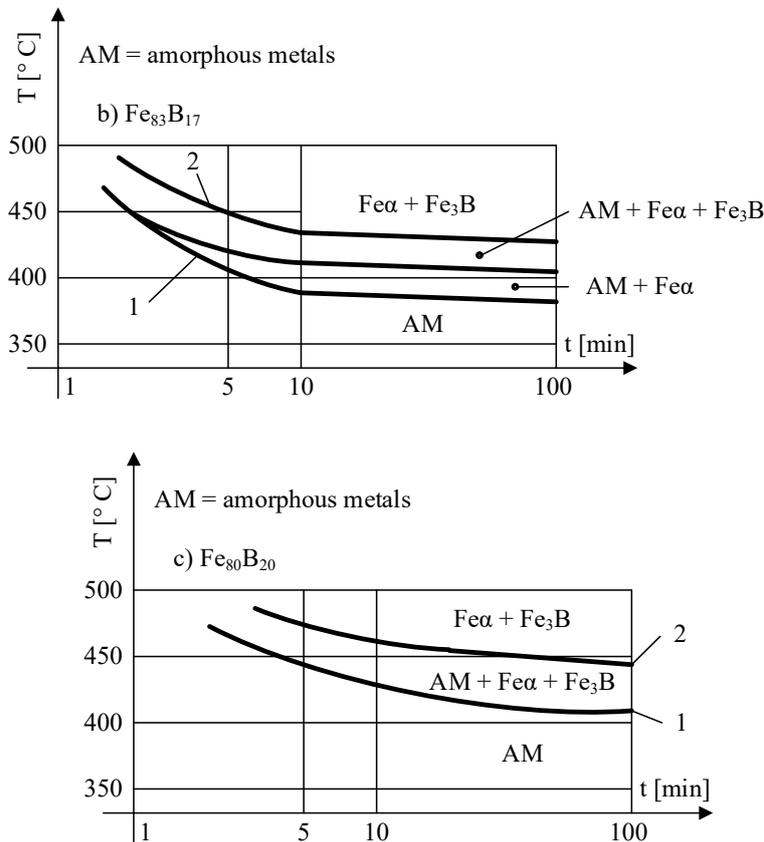
Fig. 8 TTT diagrams of alloys in the Fe-B system [9].
