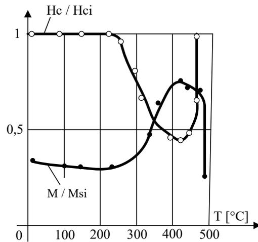
Fig. 2 The determination of the crystallization temperature in the case of the amorphous alloy  $\text{Fe}_{76.5}\text{B}_{17}\text{Si}_5\text{C}_{1.5}$  [9]
