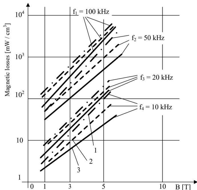
Fig.4 The influence of heating environment on the magnetic losses of an amorphous metal [9]
