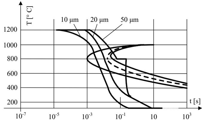
Fig. 7 TTT diagram for amorphous metal  $Fe_{83}B_{17}$  ([1], [5])
