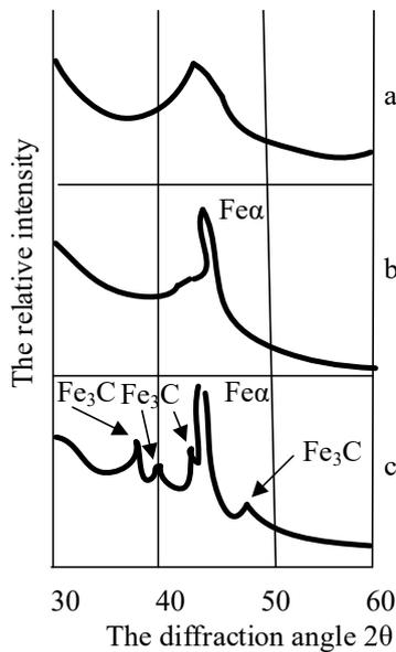
Fig. 1 The influence of heating temperature on the structure of Fe-C-O amorphous metal [9]
