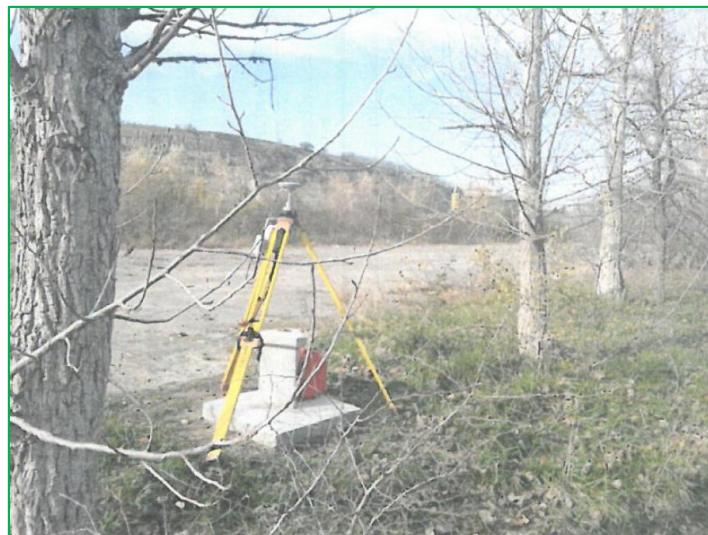
Figure 8 - Base station located in the Cemavoda area
