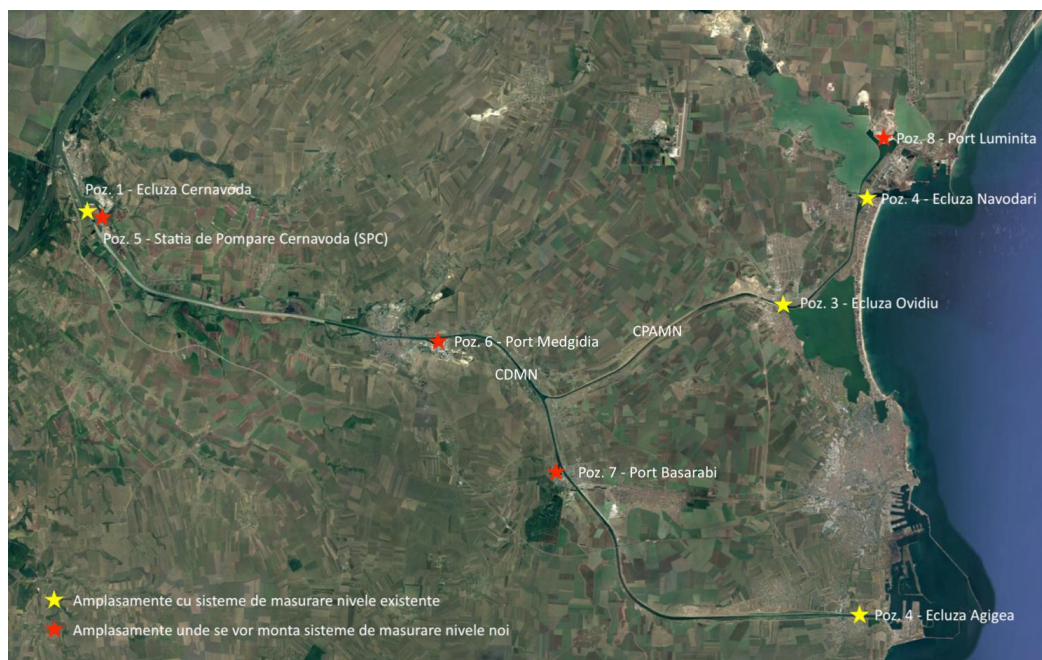
Figure 3 - Outline of water level measurement systems along CDMN and CPAMN
