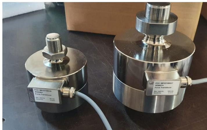
**Figure 8.** Load transducer 5 tf and 10 tf [4]
