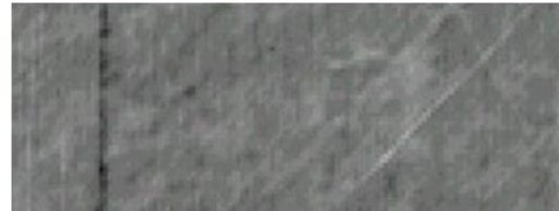
Detail 1.9. (F=143 daN; n=5; without lubrication)
