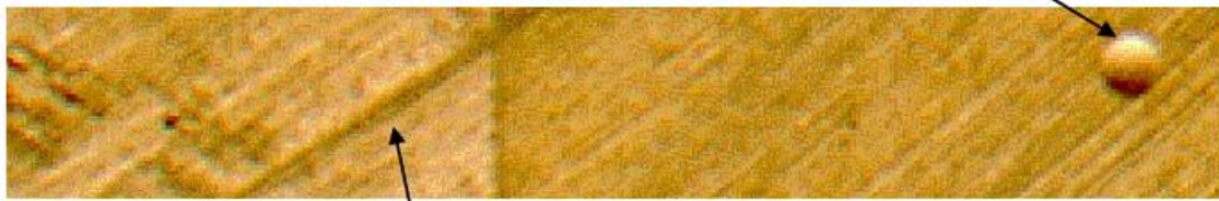
z.n.f. .. ^ Detail 2.5 (F = 328.5 daN; n = 1; with lubrication)
