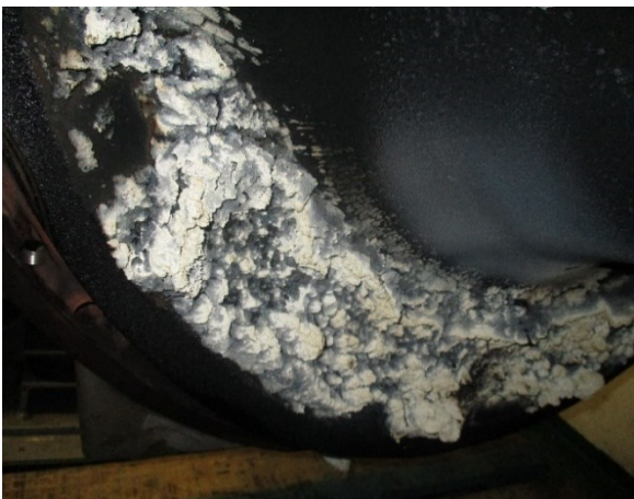
Figure 5. Contamination with unburnt oil, carbon, water.
