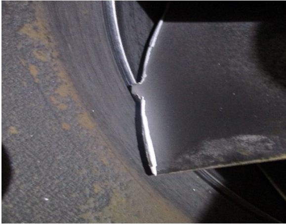
Figure 3. Compressor Wheel- found severely rubbed.
