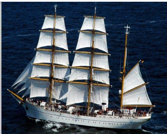
Figure 5. The yards are braced sharp in the starboard side
