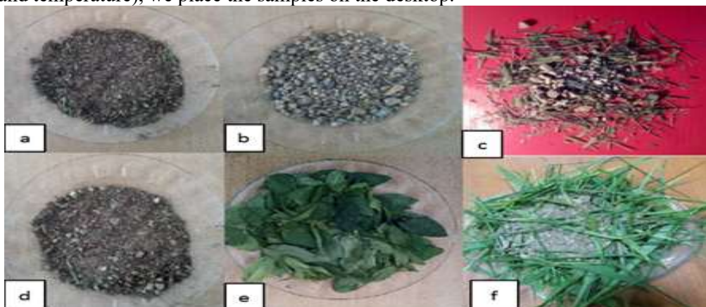
Figure 4. Materials used in the laboratory for spectroscopy; a- soil, b- sand, c- composition of grass and sand on red background, d- combination of soil and sand, e- broadleaf, f- combination of soil and grass.
