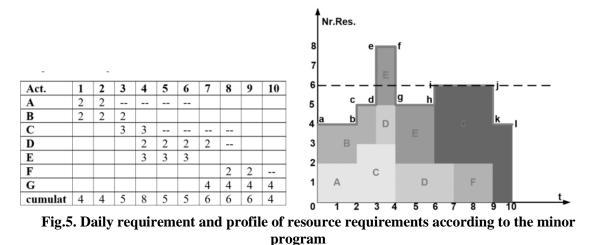
Contour a-b-c-d-e-f-g-h-i-j-k-l represents the profile of the necessary technicians, starting from the initial event to the final event. Considering that the availability of this type of resource is 6 (dotted line), it is necessary to level the allocation of the resource, if allowed, or to reschedule the activities.
