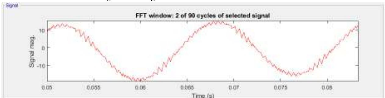
**Figure 3.** Current waveform without harmonic filters
