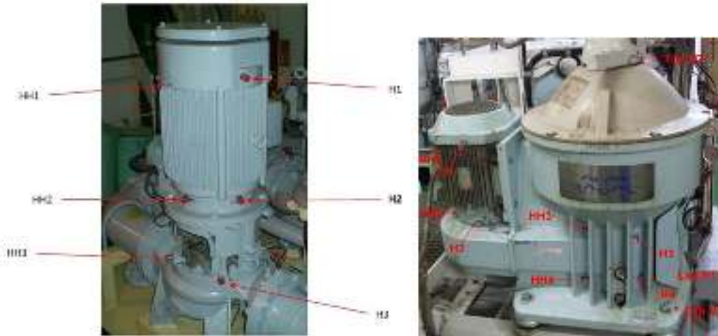
Figure 6. Vibration measurement points in the case of vertical devices and separator
