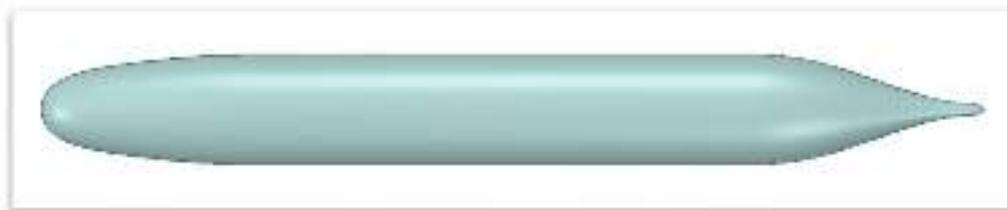
Figure 2. Modelled DARPA Suboff submarine hull
