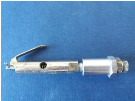
Fig. 7 The 1 st version piston with cylindrical orifice [8]
