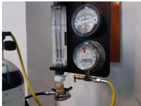
Fig. 9 Second stage regulator testing [8]
