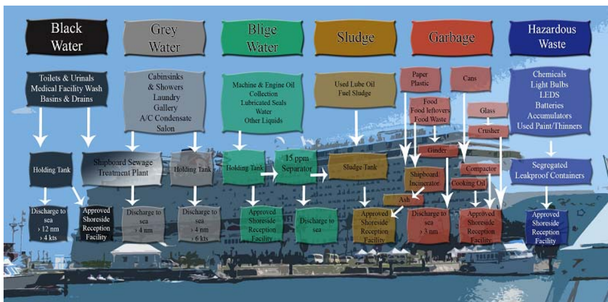
Fig.1. Complex waste handling system used on the luxury cruise liners (resource: personal & http://maritimesolutions.co.uk/ )
