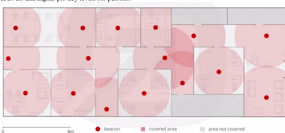
Figure 2 Example of distributing Bluetooth beacons to cover a closed space [20]
