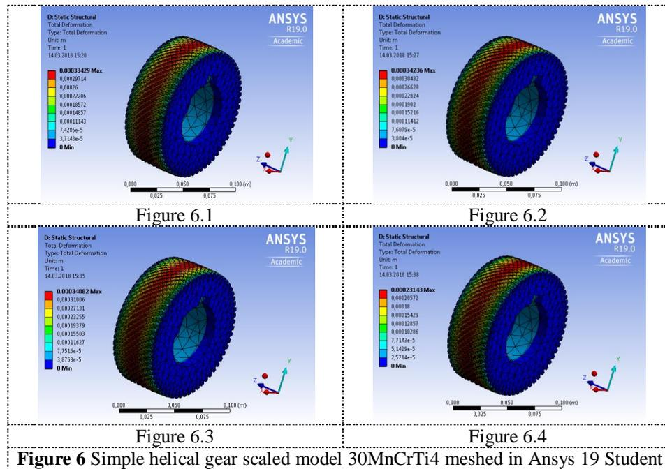
It is obvious that the deformation pattern is identical for all four working conditions and for both gear materials. The amount with which each tooth is deformed differs with the value of the  $M_2$  moment.
