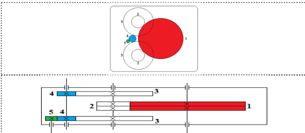
**Figure 4** Main gearbox arrangement. 1-main wheel, 2-upper and lower pinions, 3-primary wheels, 4-primary pinion for the main Gas Turbine clutch, 5-primary pinion for the Cruising Turbine clutch.
