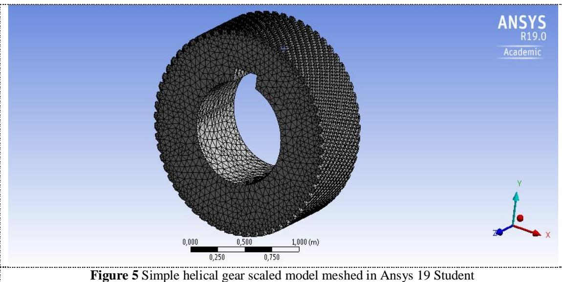
**Figure 5** Simple helical gear scaled model meshed in Ansys 19 Student
