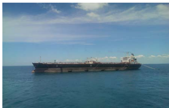
Figure 4. Tanker used for oil storage
