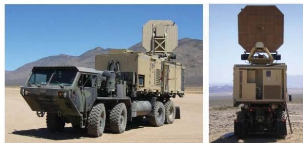
Figure 9 – ADS mounted on armored vehicles(source: https://v.wpimg.pl )
