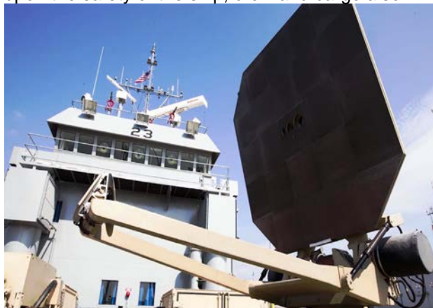
Figure 12 – ADS smaller platform mounted on a military vessel(source: https://i.ytimg.com )
