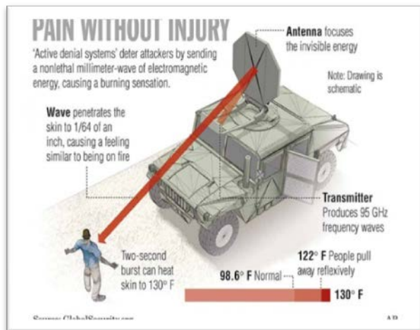
Figure 2 – Operating principle of ADS(source: https://defence.pk )
