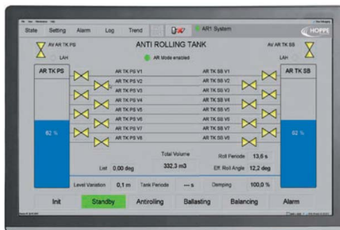
Figure 2. Antirolling passive tanks system
