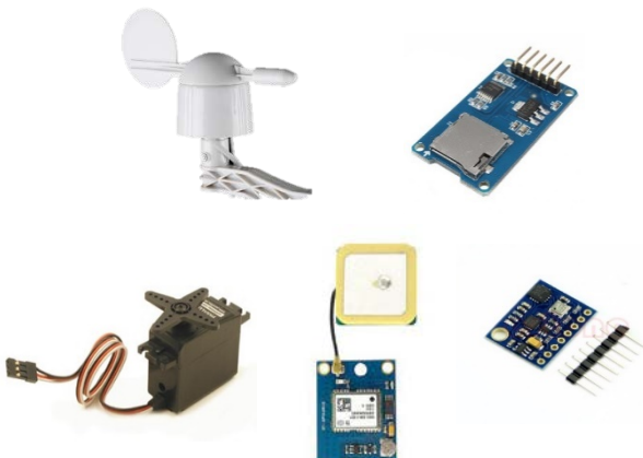
Fig. 1 - Top left Sensor: anemometer; top right sensor: SD Card Reader; botom left: Rudder Servo; botomcenter: GPS sensor; botom right: Compass sensor
