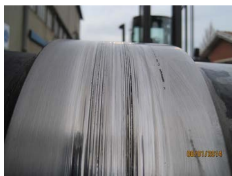
Fig.9 Upper rudder shaft bearing wear
