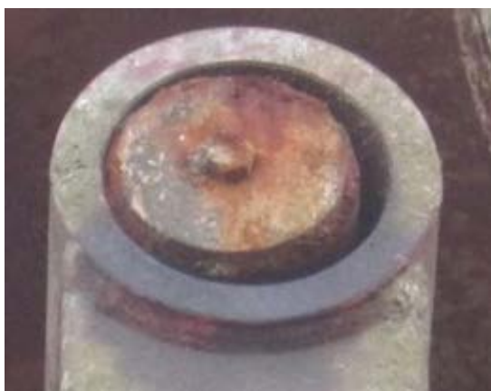
Fig. 5 The wear of the circular bearing of translation between slide and bushing guider
