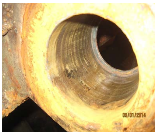
Fig.6 The bearing hole wear of antifriction alloy from fixing spur of rotated torque of the slide
