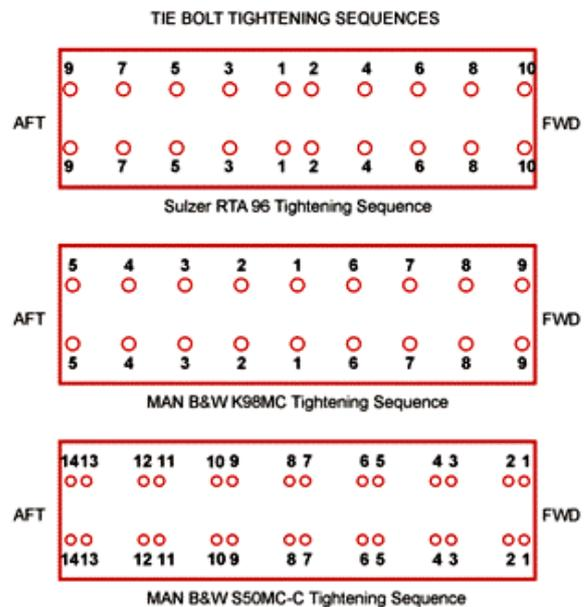
Figure 2 – The bolt tightening sequences [2, pg.44]
