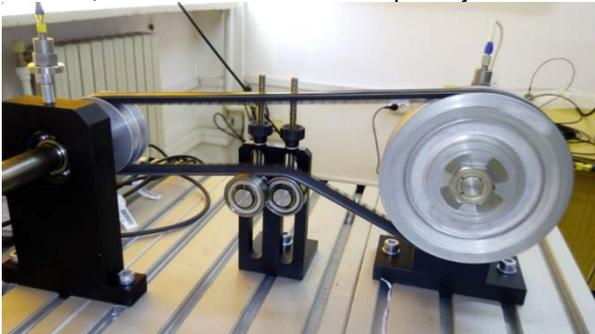
Fig.1. Mechanical belt transmission analyzed
