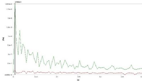
Figure 20 Time variation of minimum (red line) and maximum (green line) values of normal stress (X axis) for 18m/s impact speed
