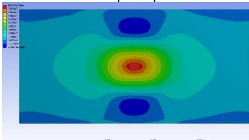
Figure 28 Distribution diagram for Normal stress (X Axis) when the maximum value is reached, for 5m/s impact speed
