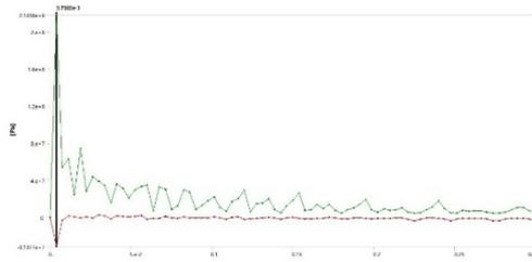
Figure 14 Time variation of minimum (red line) and maximum (green line) values of normal stress (X axis) for 12m/s impact speed
