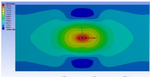
Figure 37 Distribution diagram for Normal stress (X Axis) when the maximum value is reached, for 14m/s impact speed
