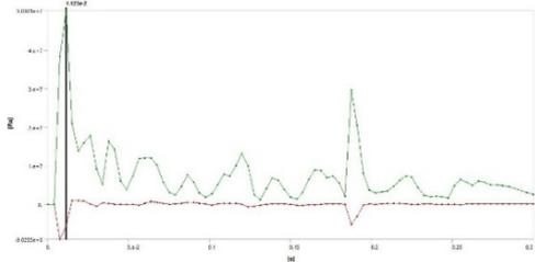
Figure 5 Time variation of minimum (red line) and maximum (green line) values of normal stress (X axis) for 3m/s impact speed
