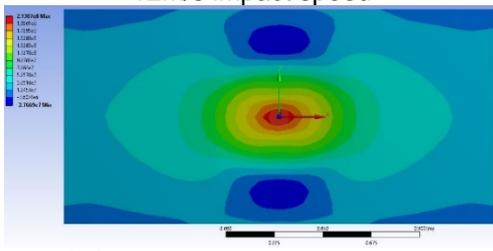
Figure 36 Distribution diagram for Normal stress (X Axis) when the maximum value is reached, for 13m/s impact speed
