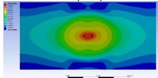
Figure 41 Distribution diagram for Normal stress (X Axis) when the maximum value is reached, for 18m/s impact speed
