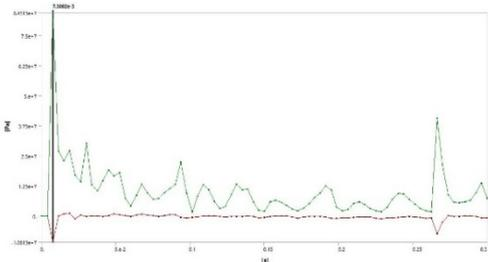
Figure 7 Time variation of minimum (red line) and maximum (green line) values of normal stress (X axis) for 5m/s impact speed
