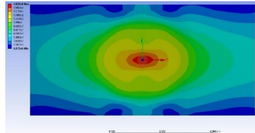
Figure 43 Distribution diagram for Normal stress (X Axis) when the maximum value is reached, for 20m/s impact speed
