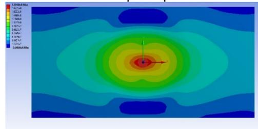
Figure 39 Distribution diagram for Normal stress (X Axis) when the maximum value is reached, for 16m/s impact speed
