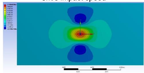
Figure 32 Distribution diagram for Normal stress (X Axis) when the maximum value is reached, for 9m/s impact speed
