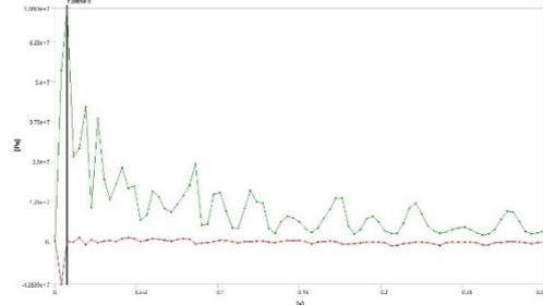
Figure 8 Time variation of minimum (red line) and maximum (green line) values of normal stress (X axis) for 6m/s impact speed
