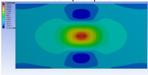
Figure 35 Distribution diagram for Normal stress (X Axis) when the maximum value is reached, for 12m/s impact speed
