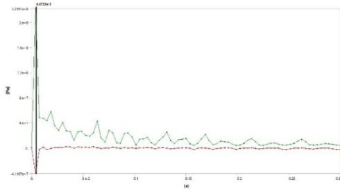
Figure 12 Time variation of minimum (red line) and maximum (green line) values of normal stress (X axis) for 10m/s impact speed
