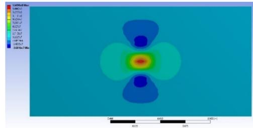
Figure 30 Distribution diagram for Normal stress (X Axis) when the maximum value is reached, for 7m/s impact speed
