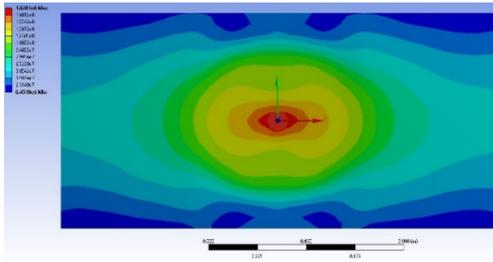
Figure 42 Distribution diagram for Normal stress (X Axis) when the maximum value is reached, for 19m/s impact speed
