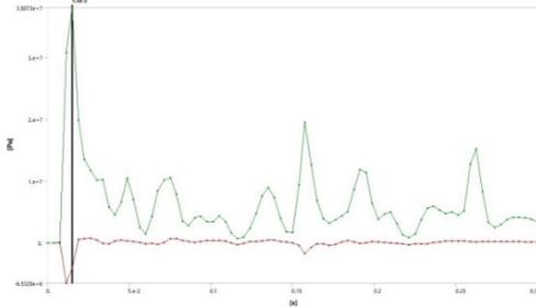
Figure 4 Time variation of minimum (red line) and maximum (green line) values of normal stress (X axis) for 2m/s impact speed
