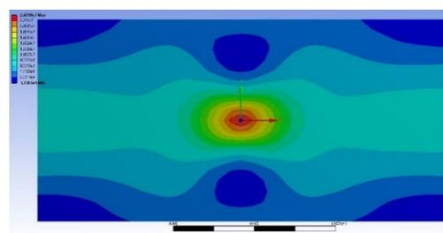
Figure 24 Distribution diagram for Normal stress (X Axis) when the maximum value is reached, for 1m/s impact speed
