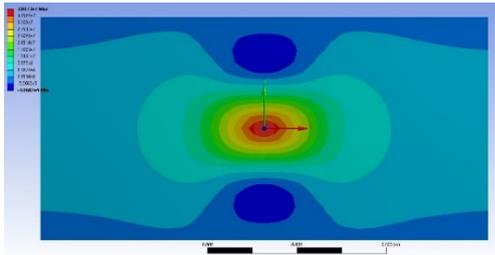
Figure 25 Distribution diagram for Normal stress (X Axis) when the maximum value is reached, for 2m/s impact speed
