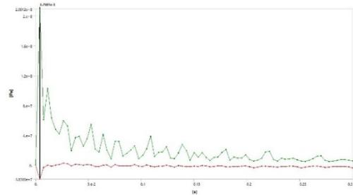
Figure 16 Time variation of minimum (red line) and maximum (green line) values of normal stress (X axis) for 14m/s impact speed
