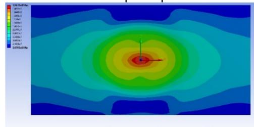
Figure 40 Distribution diagram for Normal stress (X Axis) when the maximum value is reached, for 17m/s impact speed
