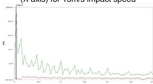
Figure 18 Time variation of minimum (red line) and maximum (green line) values of normal stress (X axis) for 16m/s impact speed
