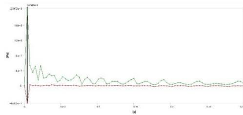
Figure 10 Time variation of minimum (red line) and maximum (green line) values of normal stress (X axis) for 8m/s impact speed
