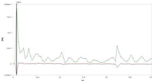
Figure 6 Time variation of minimum (red line) and maximum (green line) values of normal stress (X axis) for 4m/s impact speed
