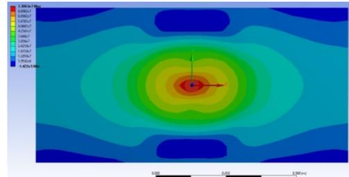
Figure 29 Distribution diagram for Normal stress (X Axis) when the maximum value is reached, for 6m/s impact speed
