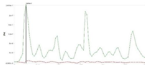
Figure 3 Time variation of minimum (red line) and maximum (green line) values of normal stress (X axis) for 1m/s impact speed
