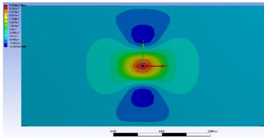
Figure 27 Distribution diagram for Normal stress (X Axis) when the maximum value is reached, for 4m/s impact speed
