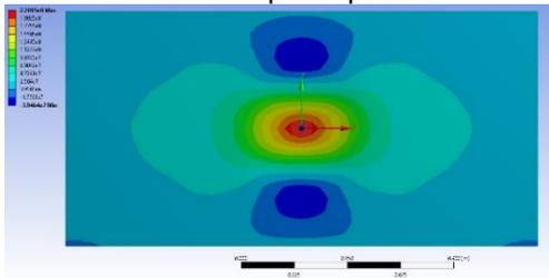
Figure 34 Distribution diagram for Normal stress (X Axis) when the maximum value is reached, for 11m/s impact speed
