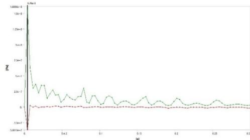
Figure 9 Time variation of minimum (red line) and maximum (green line) values of normal stress (X axis) for 7m/s impact speed
