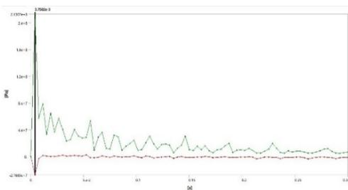
Figure 15 Time variation of minimum (red line) and maximum (green line) values of normal stress (X axis) for 13m/s impact speed
