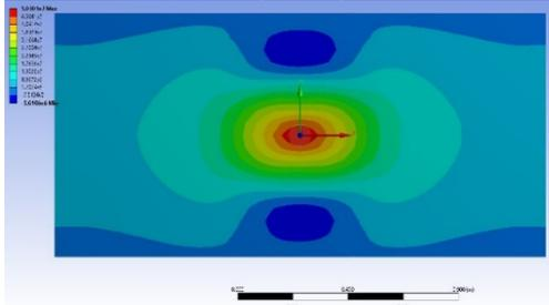
Figure 26 Distribution diagram for Normal stress (X Axis) when the maximum value is reached, for 3m/s impact speed
