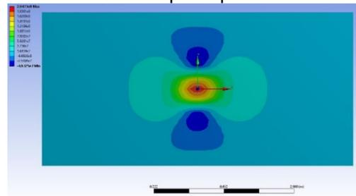
Figure 31 Distribution diagram for Normal stress (X Axis) when the maximum value is reached, for 8m/s impact speed
