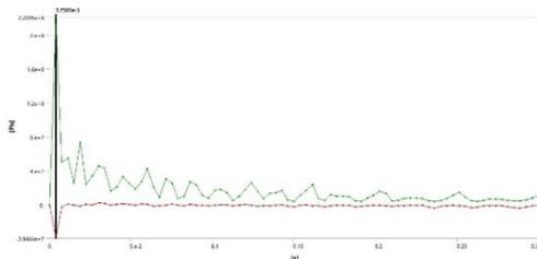
Figure 13 Time variation of minimum (red line) and maximum (green line) values of normal stress (X axis) for 11m/s impact speed
