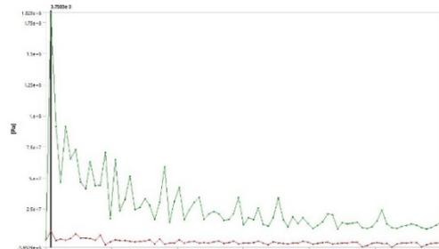
Figure 22 Time variation of minimum (red line) and maximum (green line) values of normal stress (X axis) for 20m/s impact speed
