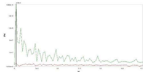
Figure 19 Time variation of minimum (red line) and maximum (green line) values of normal stress (X axis) for 17m/s impact speed
