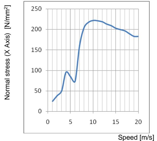
Figure 23 Variation of the maximum values for Normal stress (X Axis) depending on impact speed
