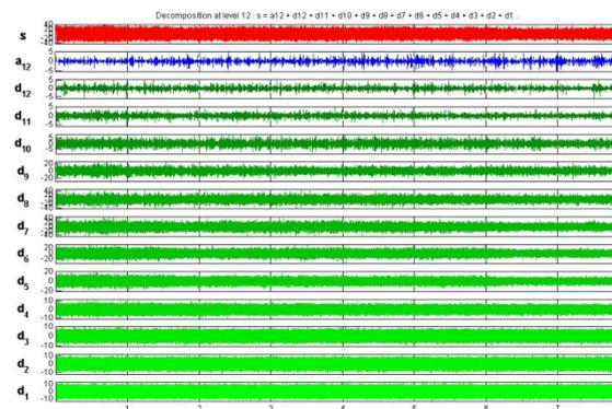
Figure 14 - DWT of Ambient noise with Ship 4 at 20m
