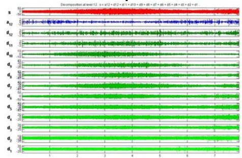
Figure 10 - DWT of Ambient noise with Ship 2
