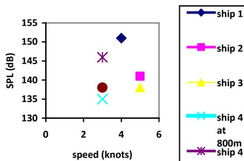
Figure 16 – Noise level vs. ship speed
