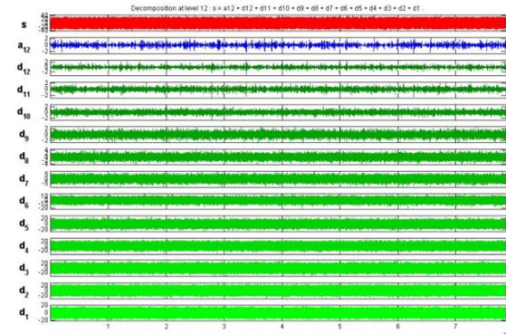
Figure 12 - DWT of Ambient noise with Ship 4 at 800m
