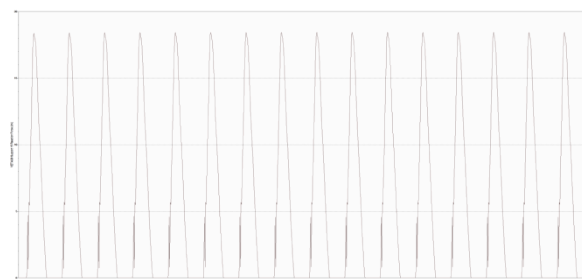
Figure 7 – Reaction force in the reversed chute maxing 18.5 kN
