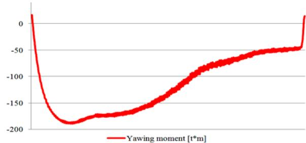
**Figure 6.** Yawing moment at 6.2 knots
