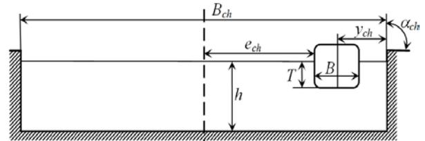
**Figure 3.** Main geometric parameters determining ship motion in a canal
