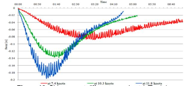
**Figure 10.** Ship sway at different speeds at  $h/T = 1.1$
