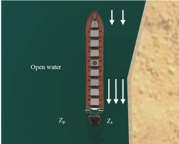
**Figure 1.** Unequal water flow caused by uneven bank wall
