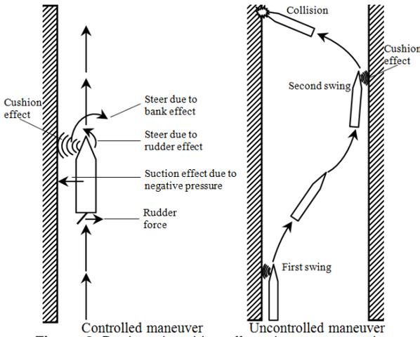
**Figure 2.** Bank and cushion effects in narrow canals
