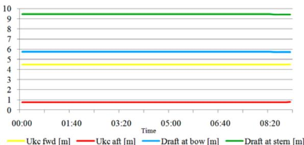
**Figure 5.** Draft and under keel clearance at 6.2 knots
