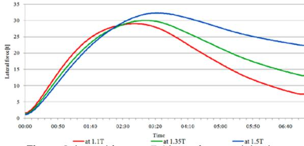
**Figure 8.** Lateral force at 7.4 knots for tested depths
