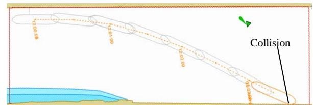
**Figure 11.** Ship track in the canal at 16 knots
