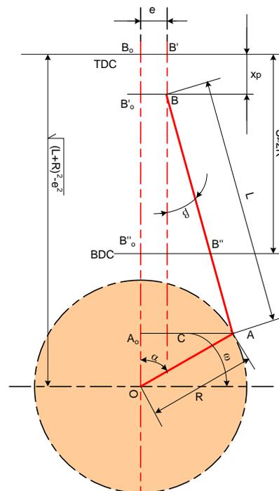
**Figure 1.3. Diagram of normal and unbalanced mechanism**
