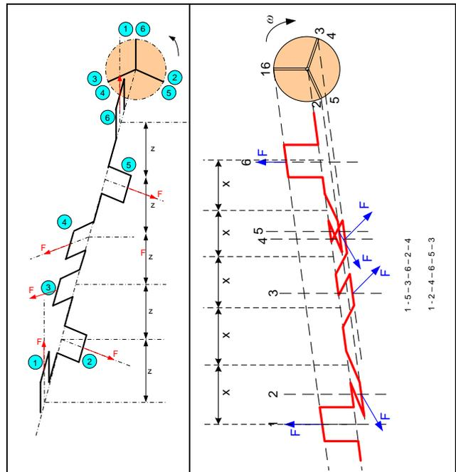
Figure 1.12. Choosing the optimal ignition order in terms of reducing the torsional vibration of the crankshaft for a 6-cylinder engine.
