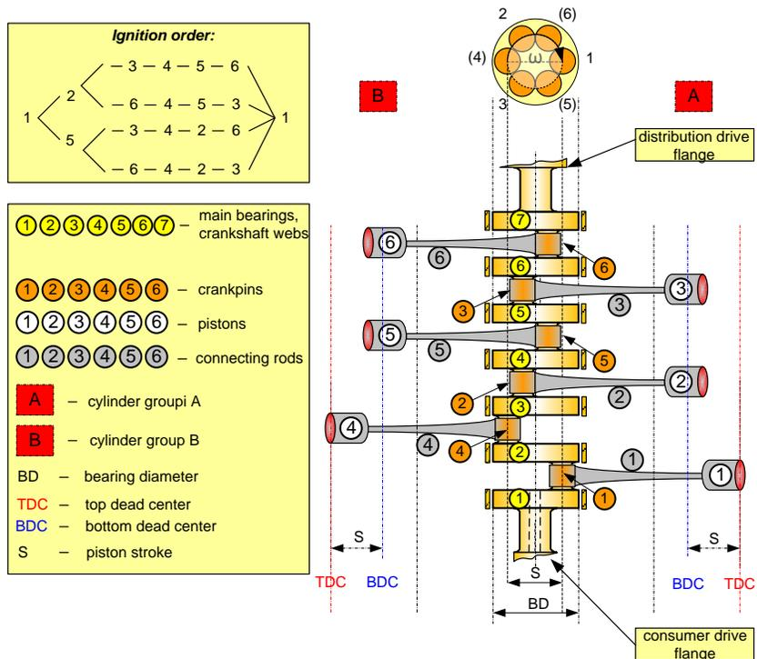
Figure 1.17. 6 cylinders, 4 stroke boxer engine configuration, constructive version.
