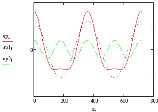
Figure 1.6. Piston acceleration diagram and his harmonics.
