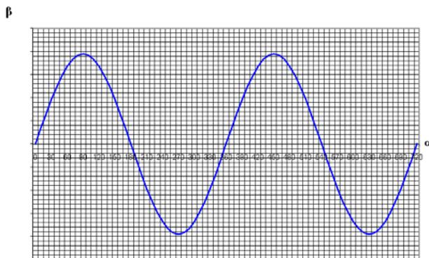
Figure 1.7. Connecting rod obliquity diagram.
