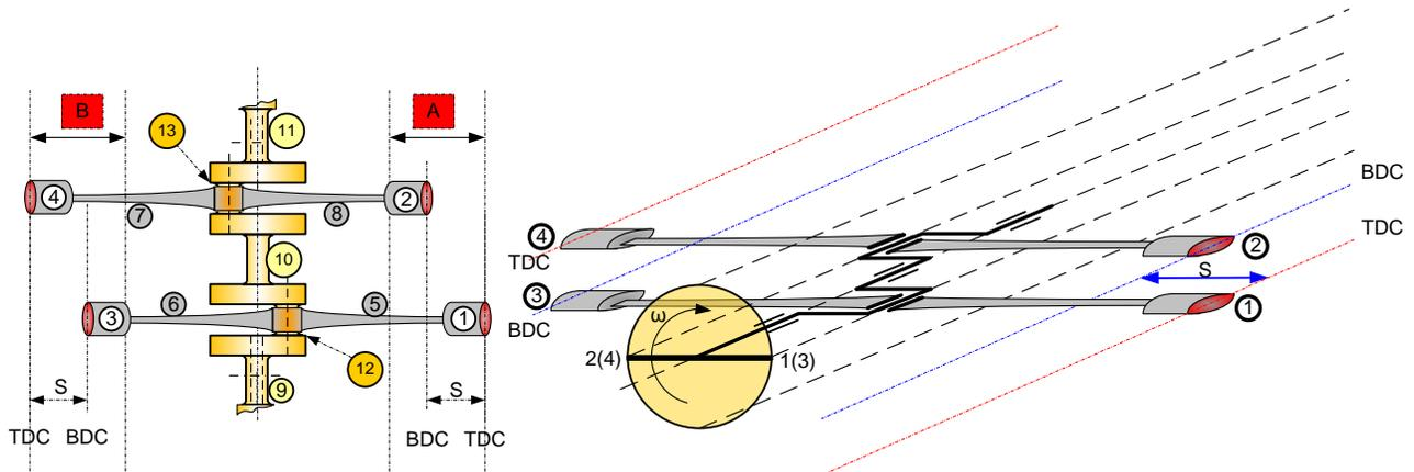
Figure 1.16. 4 cylinders, 4 stroke horizontally 180° cylinders layout V engine configuration.
