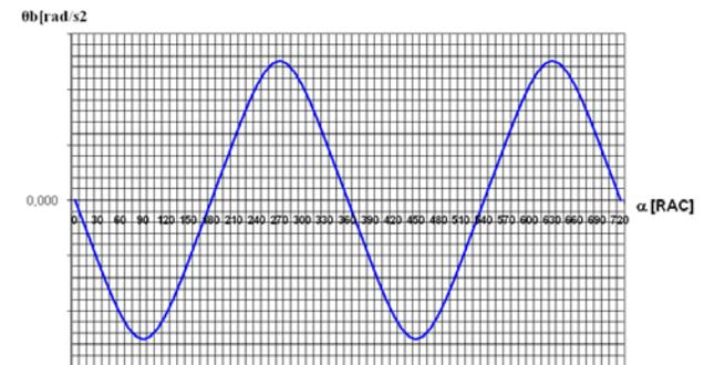
Figure 1.9. Connecting rod angular acceleration diagram.
