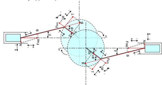
Figure 1.15. The arrangement of forces and moments in the Boxer internal combustion engine mechanism
