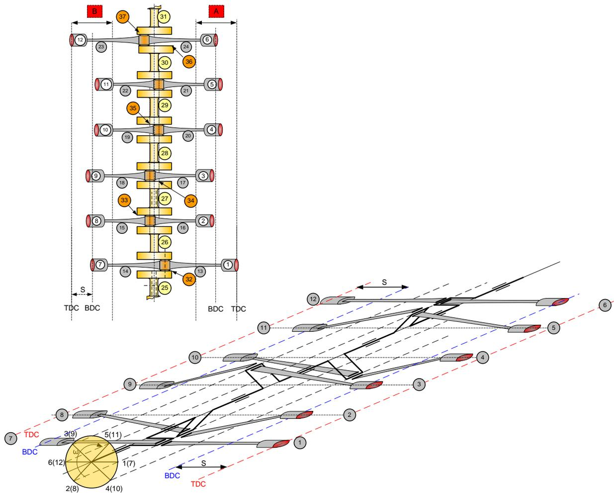
Figure 1.19. 12 cylinders, 4 stroke boxer engine configuration, constructive version:
