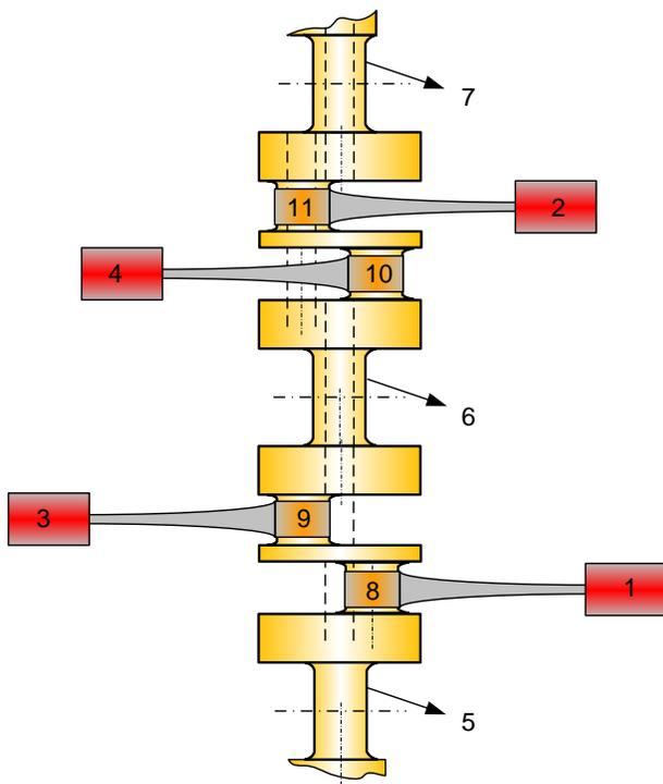
Figure 1.13. Graphical representation of the "boxer" type engine mechanism: 1,2,3,4 – pistons; 5,6,7 – main bearings; 8,9,10,11 – crankpins
