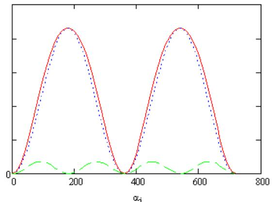
Figure 1.4. Piston movement diagram and his harmonics.
