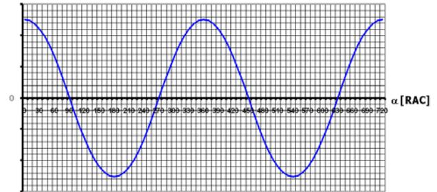
Figure 1.8. Connecting rod angular velocity diagram.
