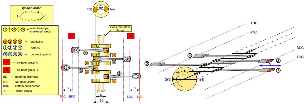
Figure 1.16'. 4 cylinders, 4 stroke boxer engine configuration, constructive version.
