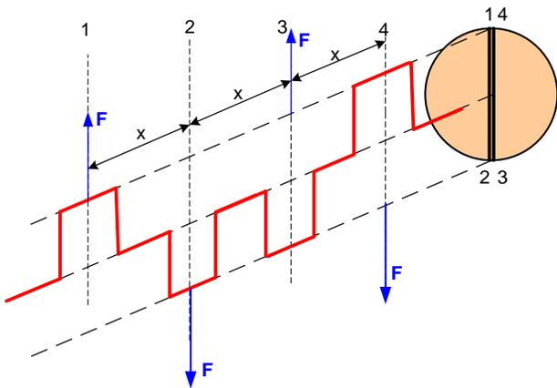
Figure 1.10. Crank plans projections on a crankshaft axis normal plan, resultant force that acting on the crankpin and the distance between crankpins.
