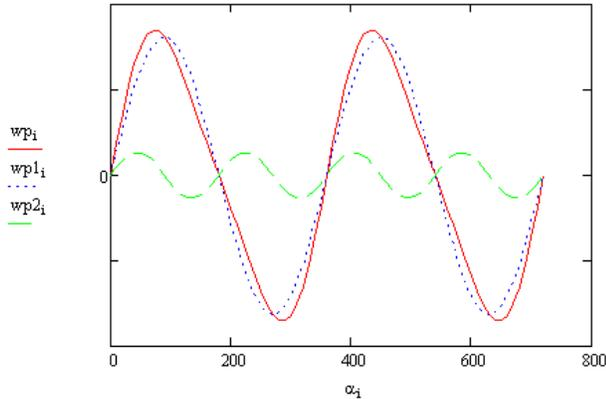
Figure 1.5. Piston velocity diagram and his harmonics.
