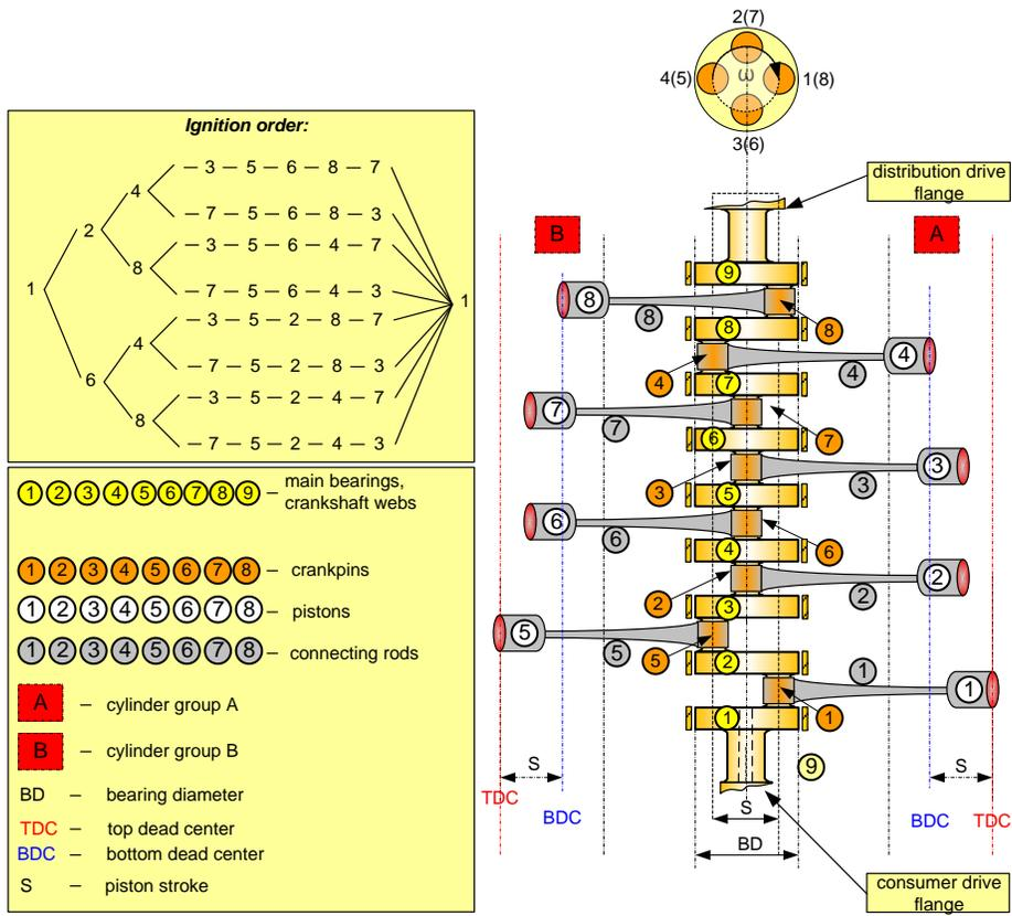
Figure 1.18'. 8 cylinders, 4 stroke boxer engine configuration, constructive version.
