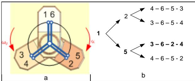
Figure 1.11.a. - Determination of crank configuration.
