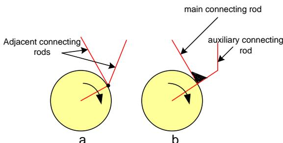
**Figure 1.2. Articulated mechanisms**
