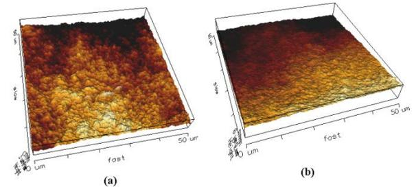
Figure 9. 3D - AFM images of epoxy resin/Zn composite coatings surface: (a) - untreated; (b) - with SRB bacteria attached and EPS formed
