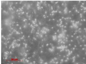
Figure 4. EFM image of the SRB attachment and EPS formed on pure zinc surface
