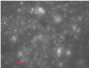
Figure 5. EFM image of the SRB attachment and EPS formed on PF resin/Zn composite coating surface
