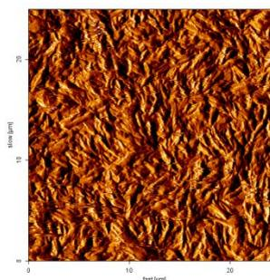
Figure 2. 2D - AFM image of untreated PF resin/Zn composite coating surface (25 $\mu$ m x 25 $\mu$ m)
