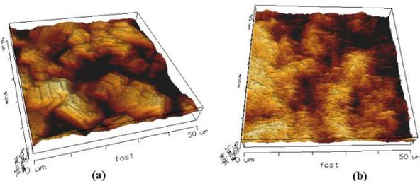
Figure 7. 3D - AFM images of pure zinc surface: (a) - untreated; (b) - with SRB bacteria attached and EPS formed
