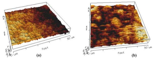
Figure 8. 3D - AFM images of PF resin/Zn composite coatings surface: (a) - untreated; (b) - with SRB bacteria attached and EPS formed
