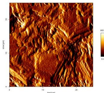
Figure 1. 2D - AFM image of untreated pure zinc surface (25 $\mu$ m x 25 $\mu$ m)
