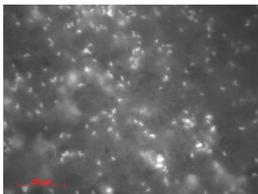
Figure 6. EFM image of the SRB attachment and EPS formed on epoxy resin/Zn composite coating surface
