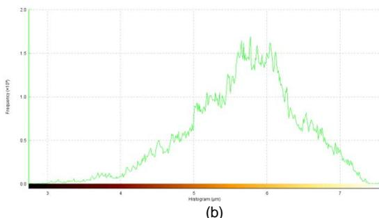
Figure 10. Histograms of the scanned surfaces for pure zinc surface: (a) - untreated; (b) - with SRB bacteria attached and EPS formed
