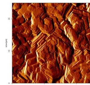
Figure 3. 2D - AFM image of untreated epoxy resin/Zn composite coating surface (25 $\mu$ m x 25 $\mu$ m)
