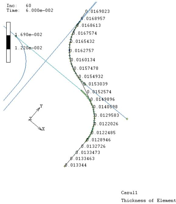
Fig. 7. Variation of thickness in longitudinal section for A steel piece
