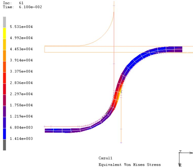
Fig. 9. Variation of tension flow after von Mises criterion, for A steel piece (without lubricant)
