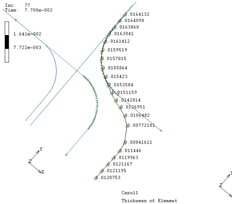
Fig.11. Variation of thickness in longitudinal section for A steel piece (without lubricant)
