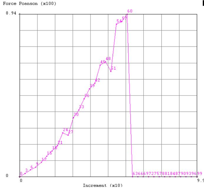
Fig. 6. The diagram force – stroke for A steel piece
