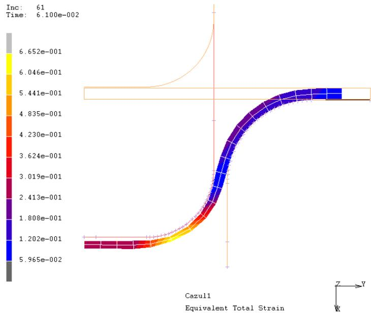
Fig. 8. Variation of total strain equivalent for A steel piece (without lubricant)
