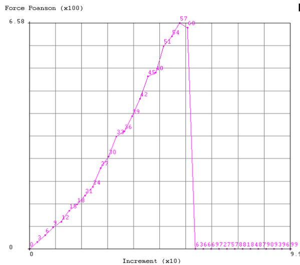
Fig. 10. The diagram force – stroke for A steel piece (without lubricant)
