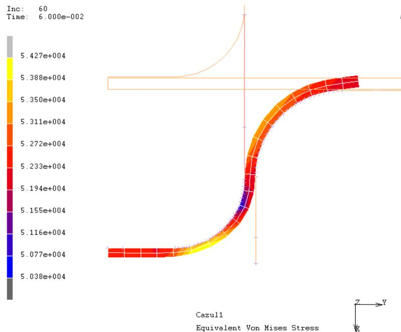
Fig.5. Variation of tension flow after von Mises criterion, for A steel piece
