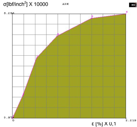
Fig. 1: The characteristic curve  $\sigma$ - $\epsilon$  for A steel introduced by points
