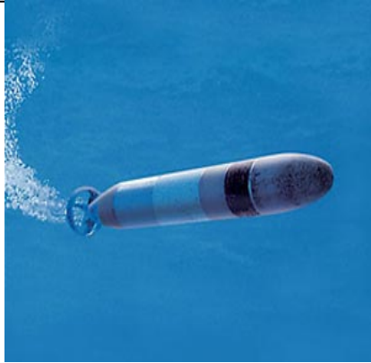
Fig. 1. The MK 39 EMATT ASW exercise target
